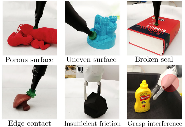
Fig. 1: Failure modes for a parallel jaw gripper and a vacuum suction cup. We define objects that result in repeated failures as sequential failure objects (SFOs) and aim to reduce the sequential failure rate (SFR) across these objects.
