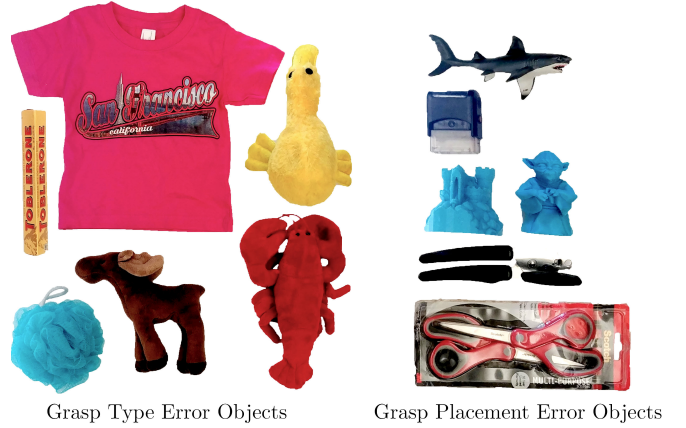
Fig. 4: 12 SFOs used to benchmark the non-Markov bin picking policies compared to the standard Markov policy. SFOs that cause grasp type errors (left) are: a Toblerone chocolate bar, a shirt, a stuffed toy duck, a loofah, a stuffed toy moose, and a stuffed toy lobster. SFOs that cause grasp placement errors (right) are: a plastic shark, a rubber stamp, a 3D printed castle model, a 3D printed Yoda figure, a can opener, and a packaged set of scissors. These objects can be compared with the Level 1, Level 2, and Level 3 objects used to benchmark the development of Dex-Net 4.0 in Mahler et al. [18].
